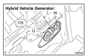
(f) Calculate the difference between the maximum and minimum resistance between terminals U – V, V – W, and W – U.
