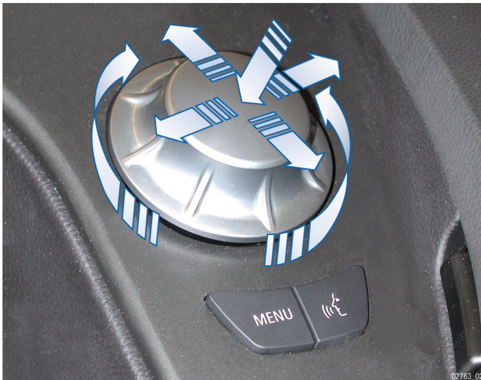
Fig. 4: E60 controller with additional control buttons (High version)
