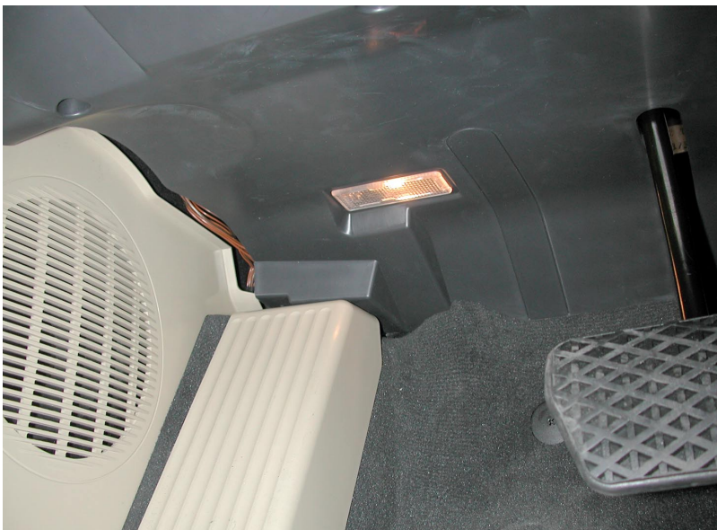
Fig. 26: E85 Installation location of woofers (low-range speakers)
