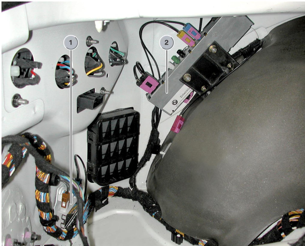
Fig. 71: E85 Installation location of aerial amplifier and aerial diversity
