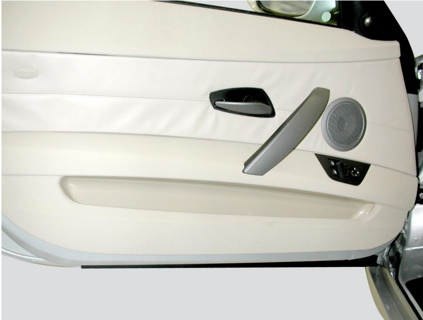
Fig. 32: E85 Front mid-range speaker in driver's door
