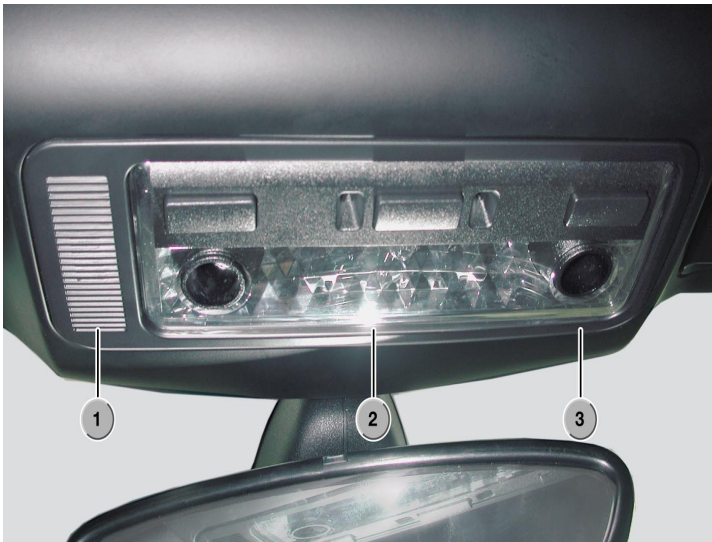
Fig. 45: E85 Installation location of the hands-free microphone
