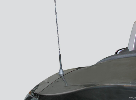
Fig. 17: E85 Installation location of rod aerial
