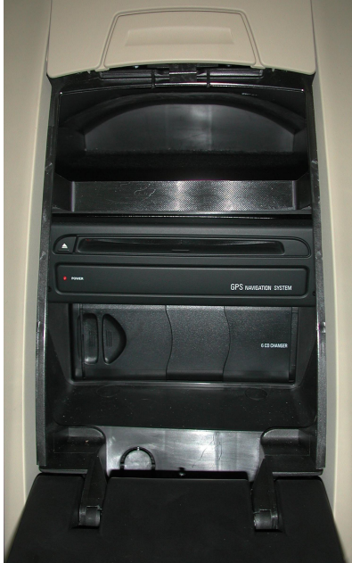
Fig. 16: Installation location of CD changer
