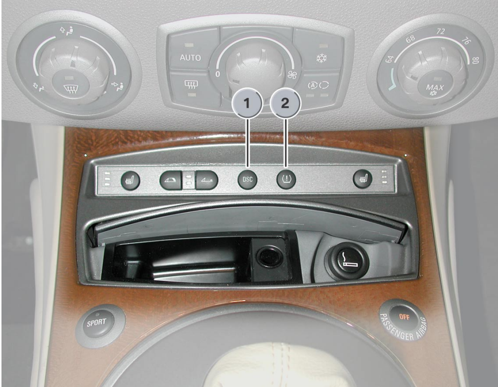
Fig. 2: E85 Installation location of DSC button
