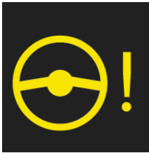
Fig. 18: Indicator lamp for EPS system in instrument cluster
