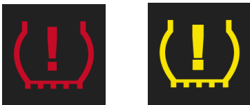
Fig. 21: RPA indicator lamp (red/yellow) in instrument cluster
