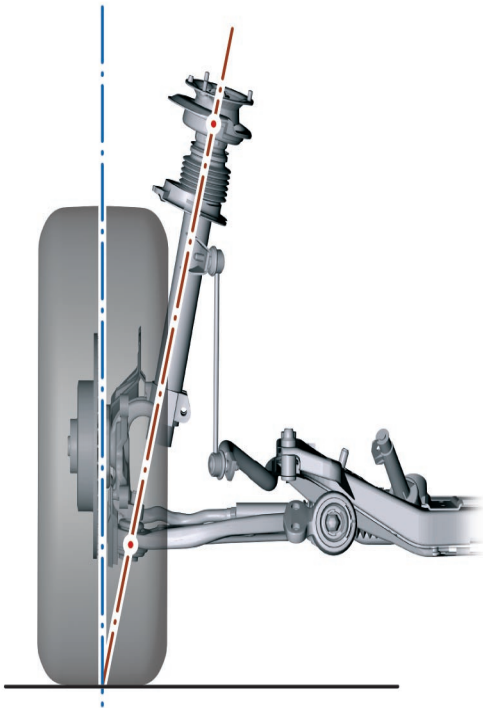
4 - Pivot axis/Steering axis
