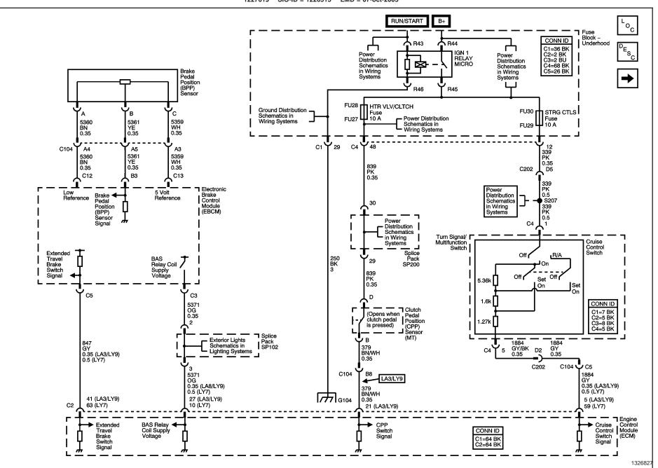
Cruise Control Schematics (Cruise Control Switch, BPP and CPP Sensors, ECM and EBCM — 2.6L/3.2L/3.6L (LY9/LA3/LY7)) SIE-ID = 1227619 SIO-ID = 1226513 LMD = 07-oct-2003
