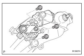
(c) Remove the 3 bolts and wiper motor.
