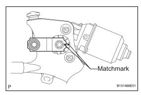
(b) Put matchmarks on the crank arm and motor, as shown in the illustration.
