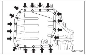
(b) Install a new gasket and the oil pan with the 18 holts
