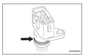
(e) Remove the O-ring from the transmission wire.
