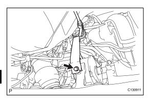
(g) Connect the clamp of the control cable with the bolt. Torque: 12 N\*m (122 kgf\*cm, 9 ft.\*lbf)
