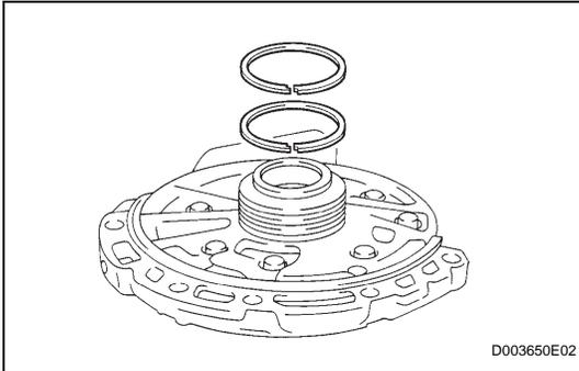
3. **REMOVE STATOR SHAFT ASSEMBLY**
