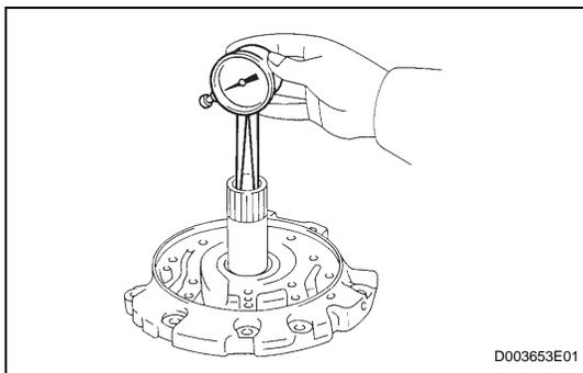
**4. INSPECT STATOR SHAFT ASSEMBLY**
