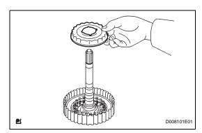
(c) Install the clutch balancer to the direct clutch drum. **NOTICE:**
