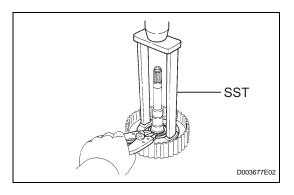
(d) Place SST on the clutch balancer and compress the piston return spring with a press.
