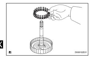
(d) Remove the piston return spring from the direct clutch drum.
