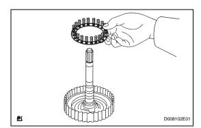
(b) Install the piston return spring to the direct clutch drum.
