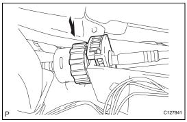
(c) Install the control cable onto the shift lever retainer.
