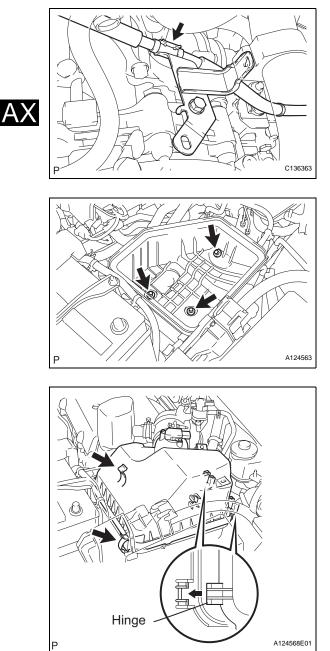
(h) Connect the control cable to the cable support.
