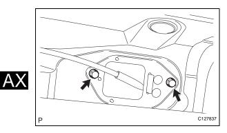
(g) Remove the 2 bolts and control cable.
