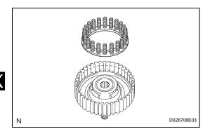
(d) Remove the forward clutch return spring from the input shaft.
