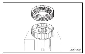
(b) Remove the flange, 5 discs and 5 plates from the forward clutch drum.
