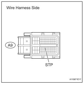
(a) Measure the voltage of the wire harness side connector. **Standard voltage**
