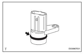
(e) Remove the O-ring from the transmission wire connector.
