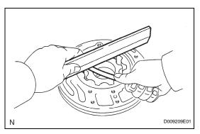
(d) Using a straightedge and feeler gauge, measure the side clearance of both gears.
