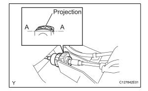
After installing, check that the lock of the cable outer is protruding beyond portion A-A, as shown in the illustration.
