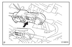
(c) Connect the control cable to the shift lever. **NOTICE:**
