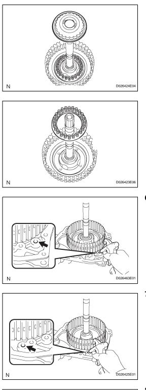
(c) Remove the clutch balancer from the direct clutch drum.
