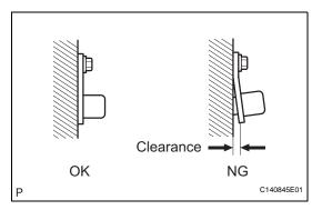
(a) Check the speed sensor NC installation.
