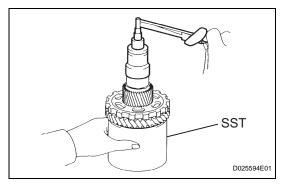
(b) Using SST and a torque wrench, measure the turning torque of the underdrive planetary gear in place while rotating the torque wrench at 60 rpm.
