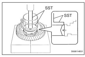
(c) Using SST a press, press in the outer race of the tapered roller bearing.
