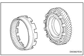
(b) Remove the underdrive planetary ring gear from the counter driven gear.
