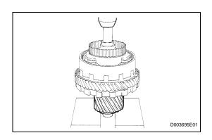
(e) Using a press, press in the differential drive pinion. **NOTICE:**
