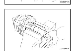
(c) Using SST, remove the lock nut. **SST 09387-00050**
