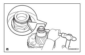
(b) Using a pin punch and a hammer, stake the lock nut.
