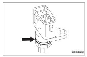
(e) Remove the O-ring from the transmission wire.
