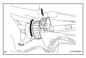
(f) Turn the nut and disconnect the control cable from the shift lever retainer.
