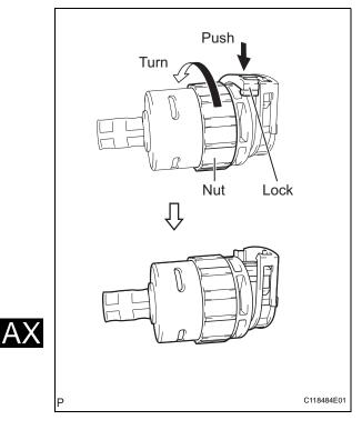
(b) Turn the nut of the control cable and push in the lock.
