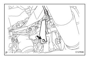
(g) Connect the clamp of the control cable with the bolt. Torque: 12 N\*m (122 kgf\*cm, 9 ft.\*lbf)
