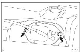
(g) Remove the 2 bolts and control cable.
