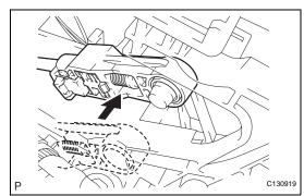
• After installing, check that the lock of the cable outer is protruding beyond portion A-A, as shown in the illustration.
