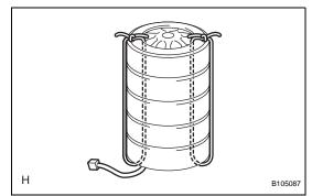
Always tie down the front seat side airbag with the airbag deployment direction facing inside the tire.
