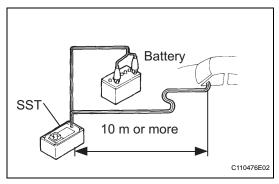
(2) Press the SST activation switch, and check that the LED of the SST activation switch illuminates.
