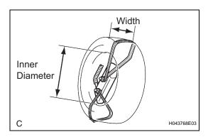
(c) Using a service-purpose wire harness for the vehicle, tie down the front seat side airbag to the tire.
