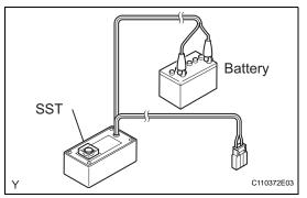
(1) Connect the SST's red clip to the positive (+) battery terminal and the black clip to the negative (-) battery terminal. HINT:
