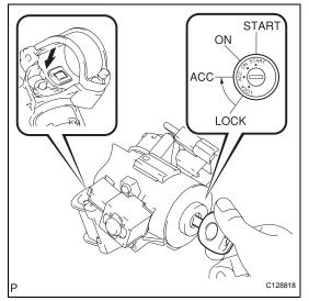
(b) Insert the key, turn the ignition switch ON (ACC) and check that the steering lock function is deactivated.
