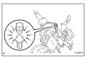
(b) Install the steering column upper with switch bracket and steering column clamp upper with new steering lock set bolt, and then tighten the bolts until their heads come off.
