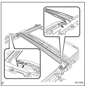
(b) Engage the 2 claws and install the sliding roof drip channel.
