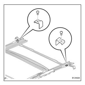
(c) Install the 2 sliding roof side stoppers with the 2 screws.
