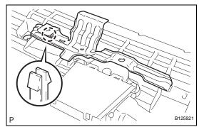
(b) Attach the claw and install the sliding roof drive gear bracket.
