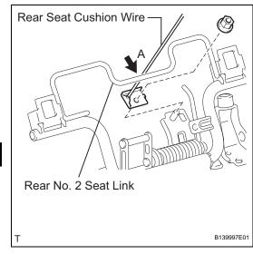
Pass the rear seat cushion wire underneath the rear No. 2 seat link part labeled A.
