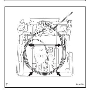
(b) Clamp the cables to the seat cushion spring with 4 new cable ties as shown in the illustration.
