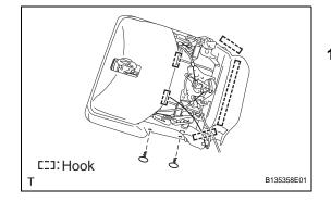
(a) Using hog ring pliers, install the seat cushion cover to the seat cushion pad with 5 new hog rings.
