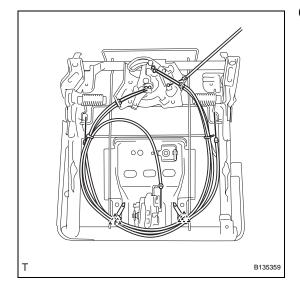
(c) Using a screwdriver, detach the hooks and remove the seat cushion cover (with pad) from the seat cushion spring.
