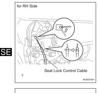
(c) Disconnect the seat lock control cable on the RH side from the seatback as shown in the illustration.
