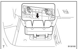
(c) Pull the hinge cover in the direction indicated by the arrow in the illustration to detach the 2 claws. Then, remove the hinge cover.
