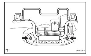
(c) Remove the 2 nuts and the rear No. 2 seat link.
