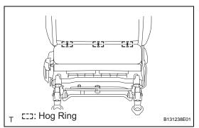
(g) w/o Seatback Board:Using hog ring pliers, install 3 new hog rings.
