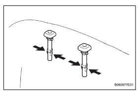
(e) Detach the 4 claws and remove the 2 headrest supports.
