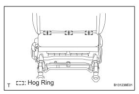
(d) w/o Seatback Board:Lift up the seatback cover and remove the 3 hog rings.
