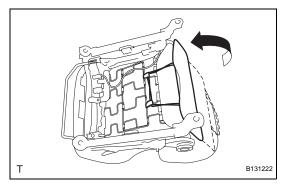
(c) Connect the 2 rubber bands of the front seatback board or front seatback cover to the seat frame (with adjuster).
