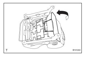
(c) Connect the 2 rubber bands of the front seatback board or front seatback cover to the seat frame (with adjuster).
