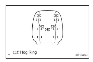
(h) Remove the 11 hog rings and seatback cover from the seatback pad.
