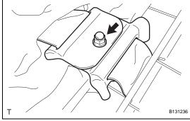
(c) w/ Front Seat Side Airbag: Fully cover the airbag with the 2 seatback cover brackets and install the nut.
