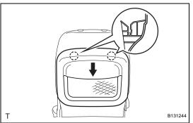
(b) Pull the seatback board in the direction indicated by the arrow in the illustration to detach the 2 claws. Then, remove the seatback board.
