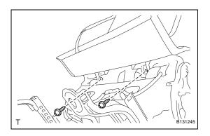
(b) Open the lower part of the seatback board. Then install the seatback board with the 2 screws.
