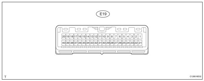
(b) Measure the voltage and resistance of the wire harness side connector.
