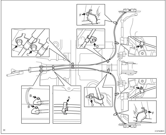
(b) Install the clamp and clamp bolt (labeled F) to the trailing arm.
