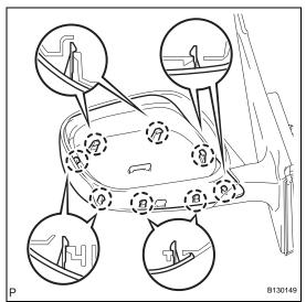
(c) Using a screwdriver, detach the 8 claws and remove the mirror cover.
