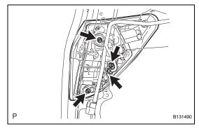
(b) Detach the clip and remove the light.
