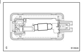
(c) Remove the light bulb from the light.
