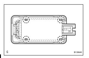
(b) Detach the 4 claws and remove the light shade.
