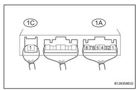
(b) Measure the resistance of the integration relay.Standard voltage
