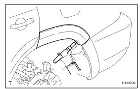
(b) Using an air riveter or hand riveter with a nose piece, strike 2 rivets to the vehicle to install the rear quarter outside moulding to the vehicle.
