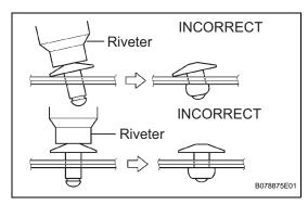
Confirm that the rivets are seated properly against the moulding. Do not tilt the riveter when installing the rivet to the moulding. Do not leave any space between the rivet head and moulding.
