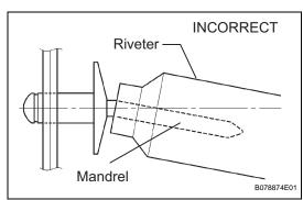
Do not pry the rivet with the riveter, as this will cause damage to the riveter and mandrel.
