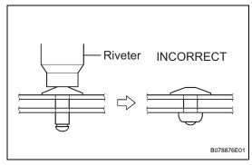
Do not leave any space between the moulding and door panel. Firmly hold together the 2 items while installing the rivet.
