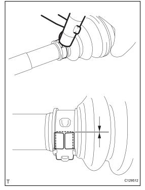
(c) Using a plastic-faced hammer, fix the buckle into place by tapping it. At the same time, use the plastic-faced hammer to adjust the lift of the lever so that the gaps between the buckle flange and lever end flange become even.
