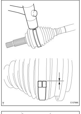
(c) Using a plastic-faced hammer, fix the buckle into place by tapping it. At the same time, use the plastic-faced hammer to adjust the lift of the lever so that the gaps between the buckle flange and lever end flange become even. NOTICE:
