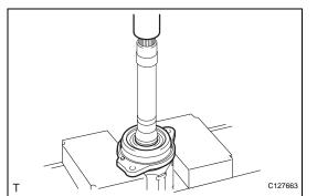
(b) Using a press, press out the drive shaft bearing case.HINT:
