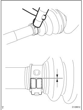
(b) Using water pump pliers, temporarily lock the boot clamp by clamping it down until a "click" sound is heard.
