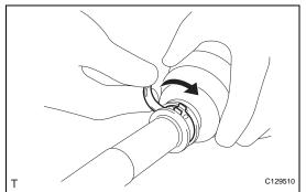
9. INSTALL FRONT AXLE OUTBOARD JOINT BOOT CLAMP LH CAUTION:
