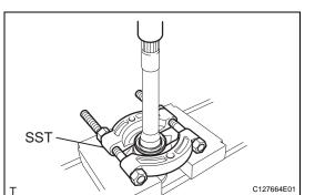
(b) Using a press, press out the drive shaft bearing case.
