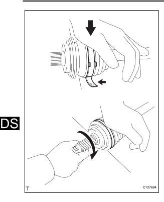
(b) With the joint on the working surface, use your body weight to press down on the joint with one hand. Then, roll the joint forward, as shown in the illustration, and press the lever in until a "click" sound is heard.
