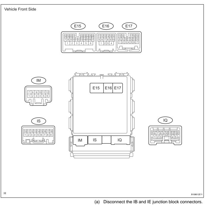
(b) Measure the resistance and voltage of the wire harness side connectors.
