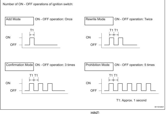
If the number of ignition switch ON - OFF operations is 0, 4, 6 or more, there will be no response (the power door lock and unlock operation) to show which mode has been selected.
