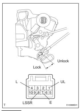
(a) Apply the battery voltage to the motor terminals and check the operation of the door lock motor.OK
