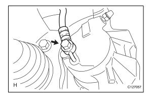
(a) Connect the flexible hose with new gasket(s) and the union bolt.
