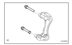
(c) Install the 2 pins (upper and lower) to the mounting.
