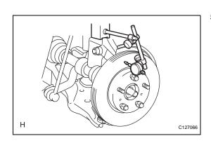
If the runout is greater than the maximum, change the installation positions of the disc and axle so that the runout will become minimal. If the runout is greater than the maximum even when the installation positions are changed, grind the disc. If the disc thickness is less than the minimum, replace the disc.
