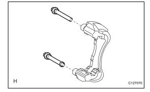
(b) Using a screwdriver, remove the slide bush from the pin (lower).
