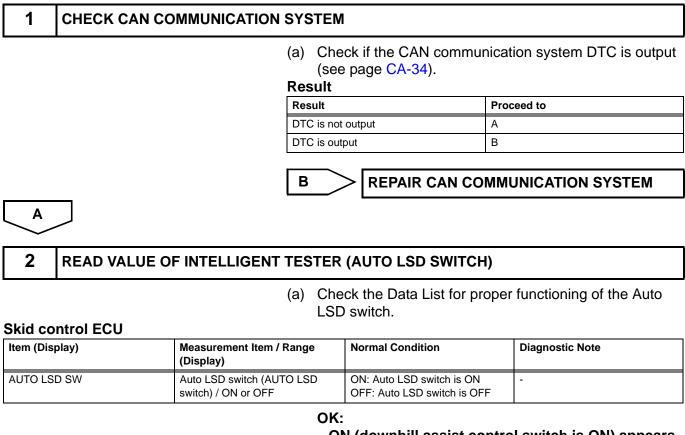
ON (downhill assist control switch is ON) appears on the screen.
