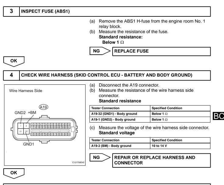
REPLACE ABS AND TRACTION ACTUATOR ASSEMBLY
